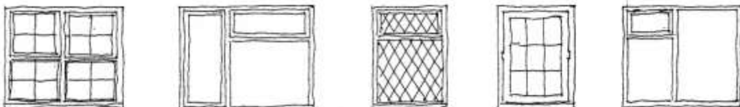
A selection of windows that do not suit for replacement in old buildings
